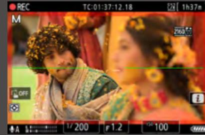
The Z 8 lets you display a red frame around the live view image on the camera monitor or viewfinder when you press the video-record button, so you know exactly, with just a glance, when you are — or more importantly, aren't — recording, to prevent mistakes.
