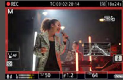
Quickly confirm and monitor your exposure with waveforms on the LCD monitor or EVF — available in two viewing sizes. You can see exactly where in the frame you might be white clipping — anytime while recording. This is especially helpful if filming in N-Log or RAW in flat colour profile when judging exposure can be difficult.
