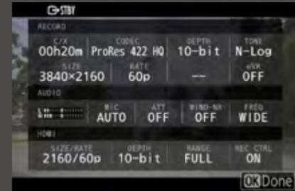
Recording settings such as the codec, on/off of electronic VR, audio, and HDMI output settings can be displayed on a single screen via the **i** menu. The top-deck control panel also displays the resolution size and frame rate along with the remaining possible recording time, so you can check that information when the camera monitor is blocked by accessories.
