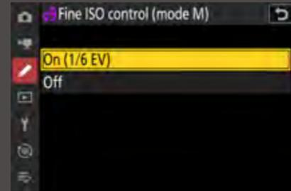
With the Z 8, you can make smooth and gradual ISO adjustments in 1/6-step increments when shooting video — useful, for example, when following a subject moving from a bright outdoor setting to a dark indoor location, and you don't want to increase the ISO more than absolutely necessary.
